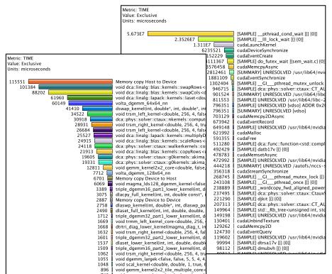
These graphs show DCA++ performance data on Summit using DCA++ for the problem size 50 and executing model beta. The graph on the left is a profile of one GPU thread, and the graph on the right is a profile of one CPU worker thread, showing considerable time spent waiting locks and semaphores. (Image Credit: TAU/RAPIDS Team)
